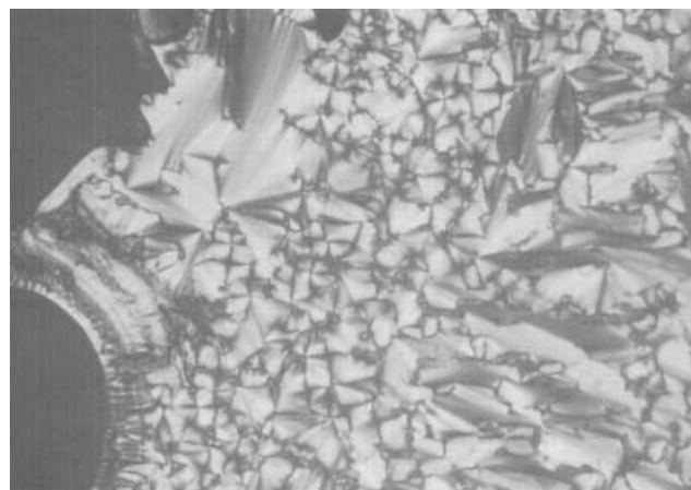
Figure 11. Contact preparation between n -nonyl gluconamide (left-hand side) and n -dodecyl 1- O - \beta -D-glucopyranoside (right-hand side), showing that the two materials are continuously miscible in their liquid-crystal phases.
