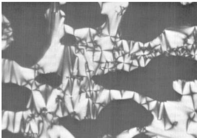
Figure 13. Coalescence of the bâtonnets of n -undecyl gluconamide to form a smectic A focal-conic texture. The formation of hyperbolic and elliptical lines of optical discontinuity can be seen clearly as black crosses in the texture.
